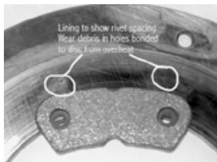
the disc, the linings should be inspected for cracking at the rivet holes. It has been reported by other brake manufacturers that in severe conditions, entire sections of the lining surface can be transferred from a severe overheat requiring immediate lining replacement.
