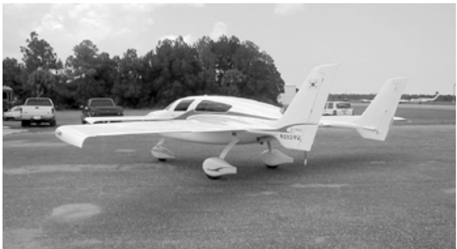
increased to 34 feet and the ailerons have been moved as far outboard as possible.
