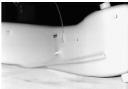
the patch over the stud. One picture shows a gear leg, and in this case the studs are to attach the gear door. Next to them is a brake hose clamp made from a nylon tie threaded through two layers of BID, about 1" square. It's best to form the hole oversize to permit later replacement.
