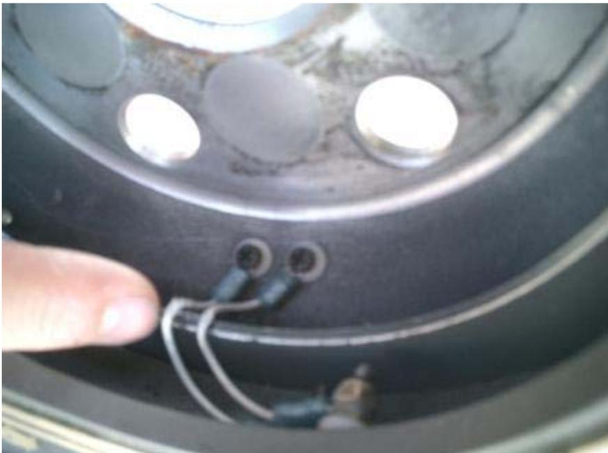
There is a brush block that rides on a ring that is attached to the starter ring gear with an electric prop. This is how the prop motor gets its power. The wires that went from the brush block ring into the starter ring gear go over a hard edge on the starter ring gear. (See Picture Below.) Both wires had chafed right at this point allowing them to short out on the starter ring gear. New wires and two little pieces of rubber tubing were all that was needed to fix this.
