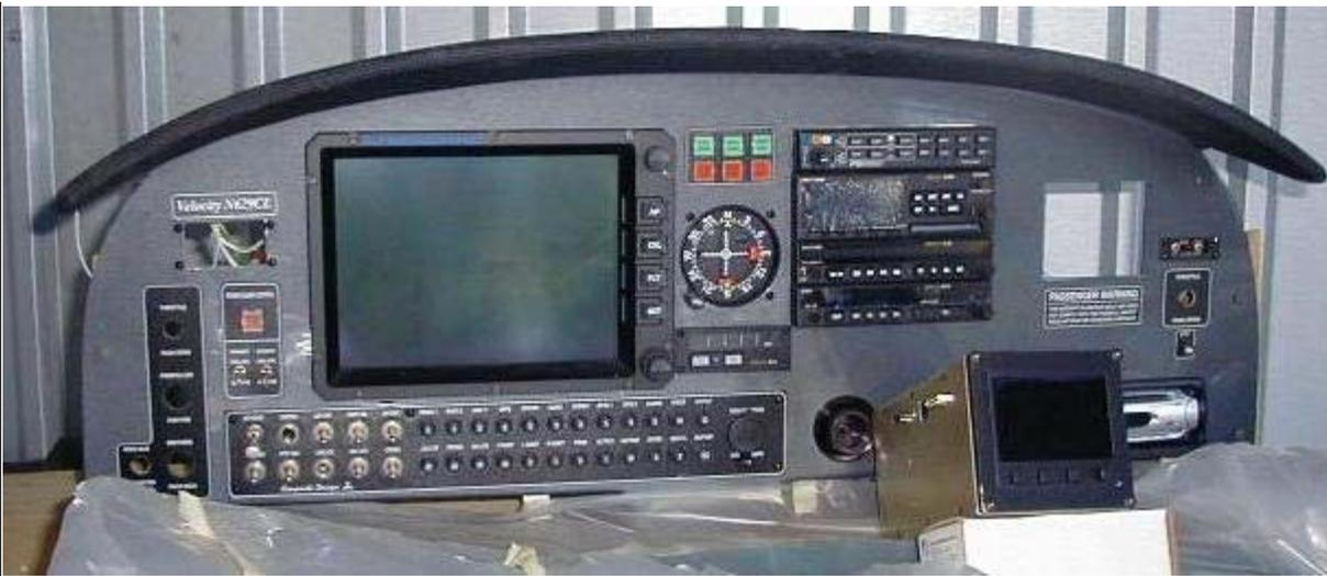
Instrument Panel painted with upholstered glare shield for Standard RG or FG aircraft.
