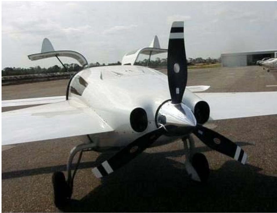
I reported in the last newsletter that Hartzell is making a two and three bladed propeller with the semi-scimitar blade design just like that used on the Cirrus aircraft. Well here it is on our XL demo airplane. We will report here when the testing is completed. Hartzell claims a 3 to 4 knot increase in speed with a better rate of climb. Time will tell.
