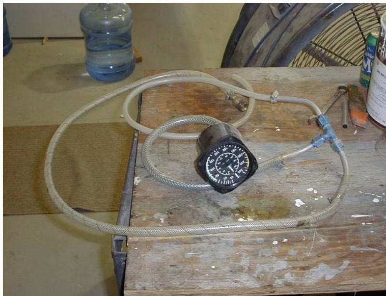
There are quite a few different types of gauges you can use with this setup. The first obvious one is a pressure gauge. Other gauges that can be used are an Altimeter or an airspeed indicator. I figure since you are building a plane these are gauges you may already have. The idea is to blow into the tube and pressurize the tank. Clamp the tube off and wait to see if the pressure bleeds off. I am satisfied when I can come back to my tank after 3-4 hours and not see a change on my gauge.
