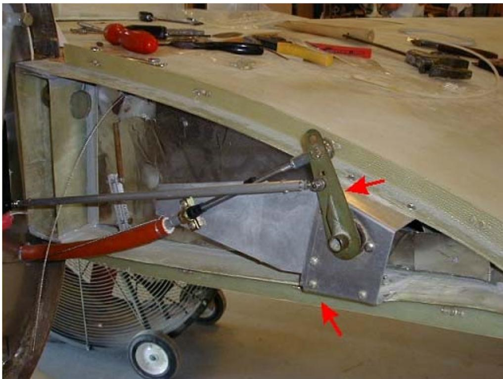
Any time you land with the brakes on or you have an unusually bad landing, It would be a good idea to check the main gear legs for cracks in the torsional wraps on the gear legs. This is more important on the retract aircraft since most of the torsional load is taken up on a smaller portion of the gear leg. This section of the gear leg is from the pivot point out about 18".
